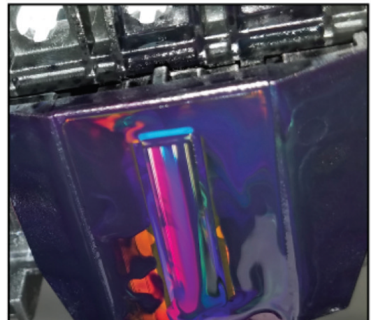
Print-head damage caused by non-HP ink (SpencerLab Digital Color Laboratory)
